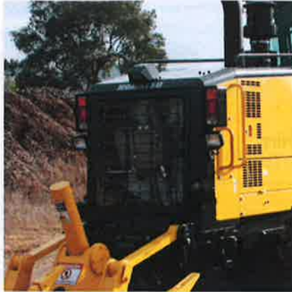
Easy radiator cleaning with reverse fan
