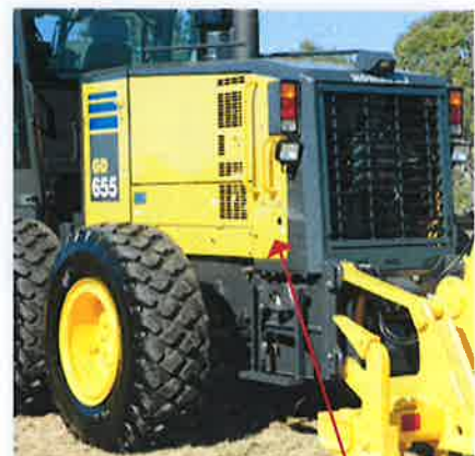
Lockable- ground level refuelling.
